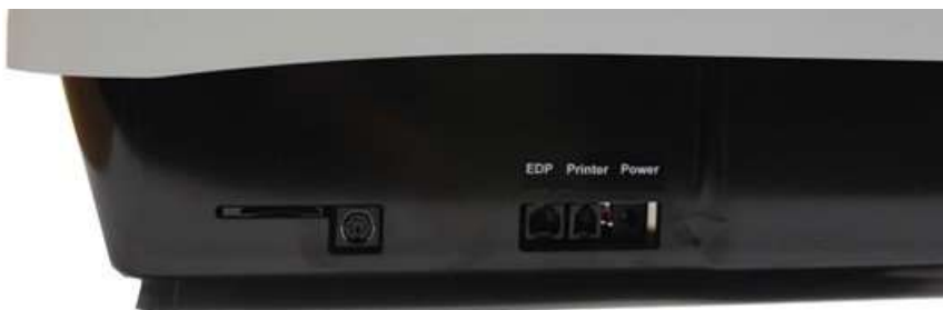
Fig. 4.1 Connections SUPER GL speedy ( EDP, Printer, Power )
