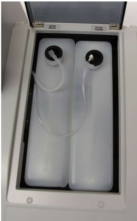
Fig. 6.3 View of supply and waste container
