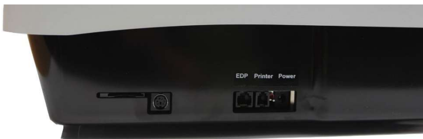
Abb. 4.1 Anschlüsse SUPER GL speedy (EDP, Printer, Power)
