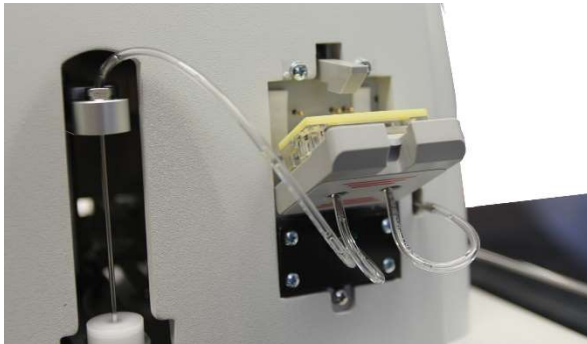
Fig. 6.2 Sensor holder open
